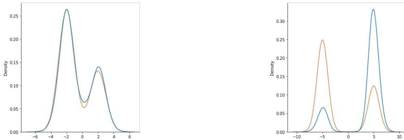
Figure 2: Training a single hidden-layer network to score match a mixture of Gaussians (ground truth green, score matching output blue) succeeds at learning the distribution when the modes are close (left, small isoperimetric constant), but not when they are distant (right, large isoperimetric constant) in which case it weighs the modes incorrectly.
