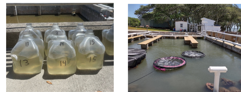
Figure 5: Algal bioassay setup in pond incubation
