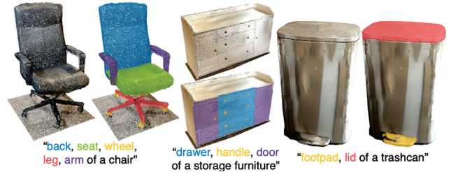
Figure 7. Each pair shows a captured point cloud by iPhone (left) and the semantic segmentation result of our method (right).
