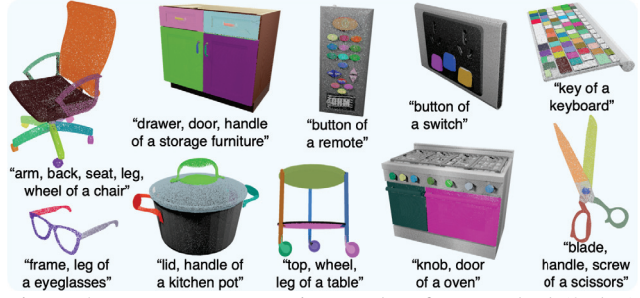
Figure 5. Instance segmentation results of our method (8-shot) on the PartNetE dataset. Different part instances are in different colors (zoom in for details).
