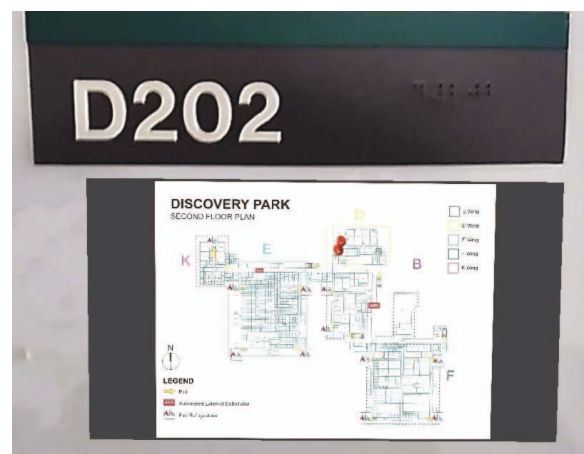
Fig. 4. The user interface of the AR mobile application
