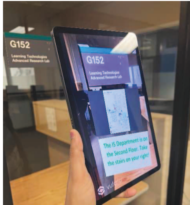
Fig. 7. View of the floor plan in the tablet triggered through a marker (room number) in the building
