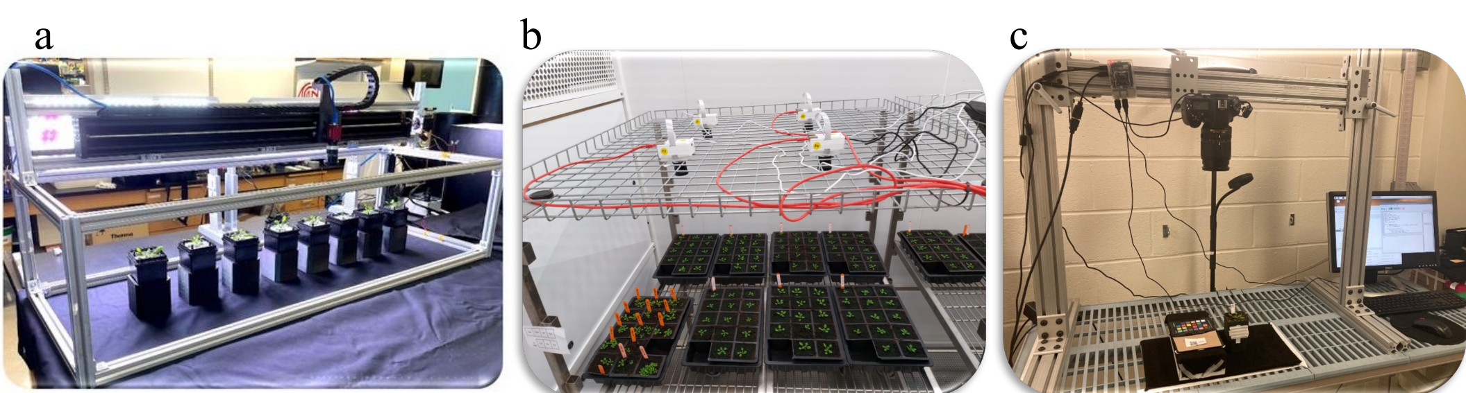
Figure 1: (a) The OPEN Leaf imaging robot developed at the DMC lab at the University of Missouri [2] using Allied Vision Mako G-503B 1/2.5" Monochrome CMOS Camera, it can capture RGB images automatically over time and upload the data to collaborators using shared online storage Cyverse [3] . (b) the Raspberry Pi imaging system used at Rothamsted Research to capture RGB top view image data; it enables the real time monitoring the growth of rosette with high resolution in growth chamber. (c) The imaging setup used at Hofstra University, developed in the Tara Enders lab using a NIKON D7200 digital cameras controlled by laptops. to A standard color palette was used to setup a reference color when comparing the color change of plant surface.
