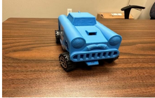
Figure 4. Final 3D printed RC car.
