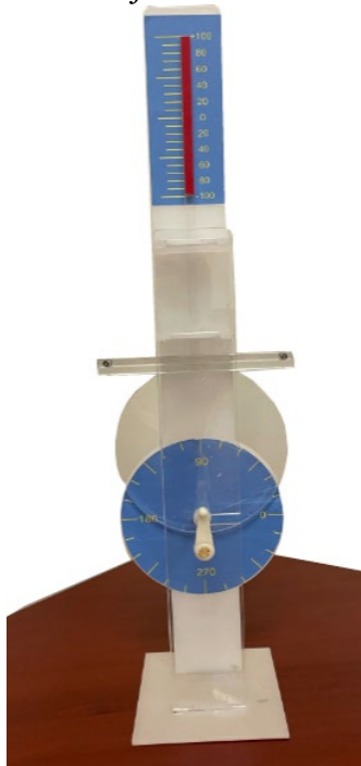
Figure 8 Isolated Rod-and-Cam Section of Wave Machine
