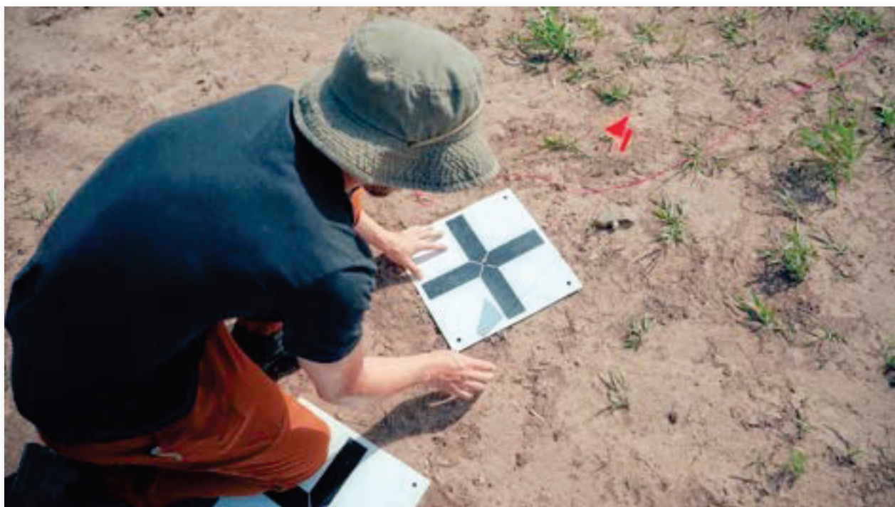
Setting up a ground control point for unmanned aerial vehicle (UAV)-based controlled experiments at Oklahoma State University's Center for Fire and Explosives (CENFEX). Note inert PFM-1 in the background.
