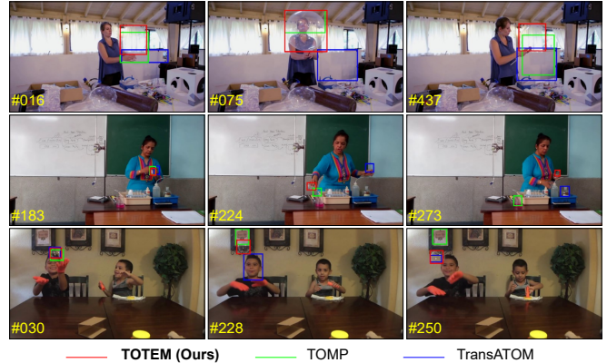
Fig. 1: Qualitative comparison of the proposed TOTEM tracking algorithm with state-of-the-arts [1], [6] on three challenging sequences from TOTB [6]. Owing to the effective fusion technique tailored for transparency awareness, TOTEM can accurately localize transparent objects under challenging scenarios. All figures in this paper are best viewed digitally, in color, significantly zoomed in.
