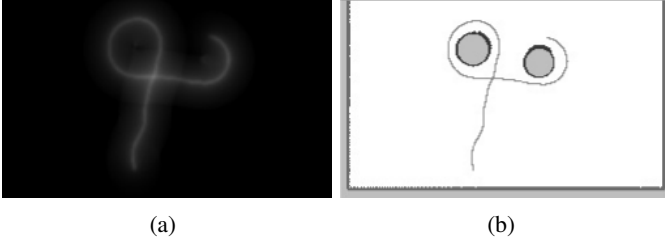
Fig. 3: A typical output of the Data Pre-processing module while a robot performs an RFID inventory task: (a) An example of m_t^v : brighter grids/pixels indicate a denser RF signal, and the tags in those grids are more likely to be scanned. (b) An example of m_t^s : black grids/pixels indicate the detected objects, grey pixels represent the unknown spaces (areas inside the black circles), and the light grey curves present the robot's navigated trajectory.
