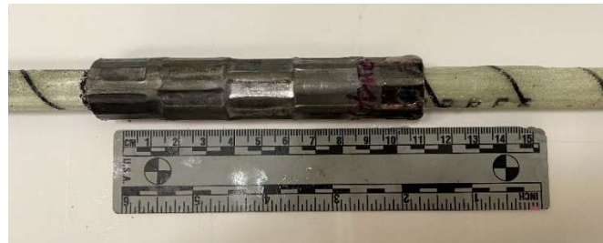
Figure 3. Spliced GFRP bars with swaged coupler
