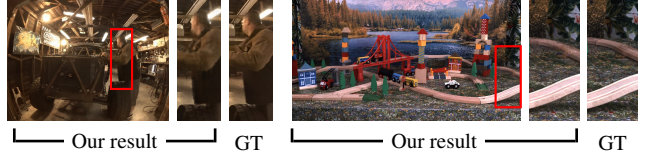
Figure 6. Limitations. Our approach can sometimes produce blurry reconstructions due to the training ray subsampling scheme (Section 3.3) (left) or noisy reconstructions in sparsely observed regions due to an under-constrained sampling network (right).
