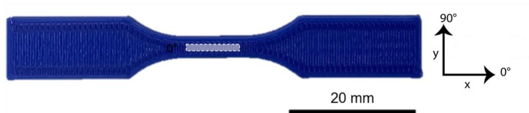
Figure 1. Image of 3D printed tensile bar using a layer thickness of 0.3 mm and 90° raster angle. The coordinate axes describe the raster angle relative to the direction of the deformation during tensile testing. The shaded box with dashed lines illustrates the area of the top surface of the printed specimens that is characterized by optical profilometry.
