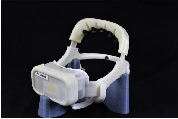
Fig. 2: NeuroEXO System: In this instantiation, we have a BCIoT platform for rehabilitation. The system is dedicated to motor imagery in a BCI application with five (EEG) electrodes across the sensorimotor cortex, three EOG electrodes, and two reference electrodes. EOG electrodes are found in the foremost arms and the front band. The deployed hardware and software can be found in the posterior area of the headset inside the white translucent box. [33]
