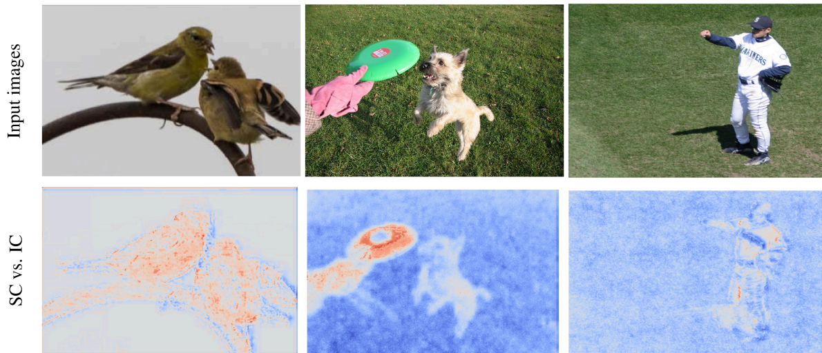
Figure 2: Bitrate comparison between a supervised compression (SC) model (Matsubara et al., 2022c) and an input compression (IC) model (Ballé et al., 2018). We plot the difference of the bits allocated for each pixel, exemplified on three images. Areas where the SC model allocates fewer and more bits for the given image are indicated in blue and red, respectively (best viewed in PDF). It is apparent how supervised compression allocates more bits to information relevant to the supervised object recognition goal.
