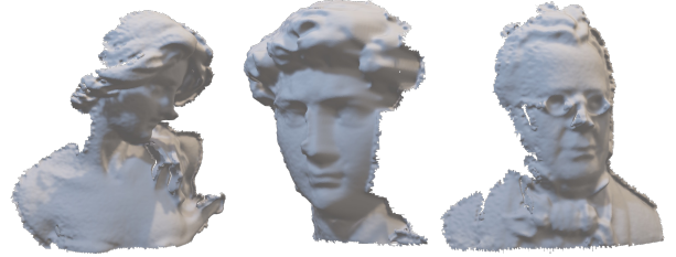
Figure 5: In simple scenes without global illumination, a single raster without global illumination suppression is sufficient. Here we present various reconstructions of opaque busts using a single 2-minute raster scan.
