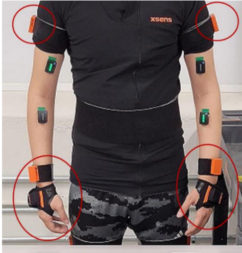
FIGURE 2: Six IMU sensors on the participant.
