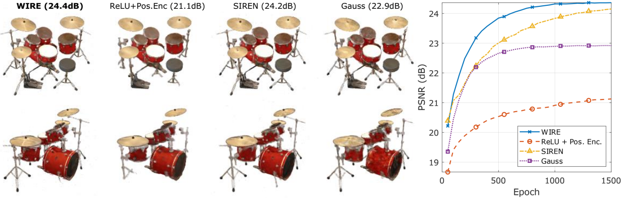
Figure 10. Novel-view synthesis with neural radiance fields. INRs have shown most promise in novel-view synthesis where the transmittance and color at each 3D voxel is modeled as output of INRs. Here, we show that WIRE is well-suited for novel-view synthesis with no additional positional encoding. WIRE not only achieves higher accuracy (+0.2dB) with fewer epochs, but captures details that are missed out by other nonlinearities, such as the rod connecting the ride cymbal to its stand and the anisotropic reflections on the cymbals.
