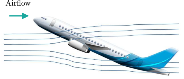
Fig. 9: Stall in a fixed-wing aircraft.
