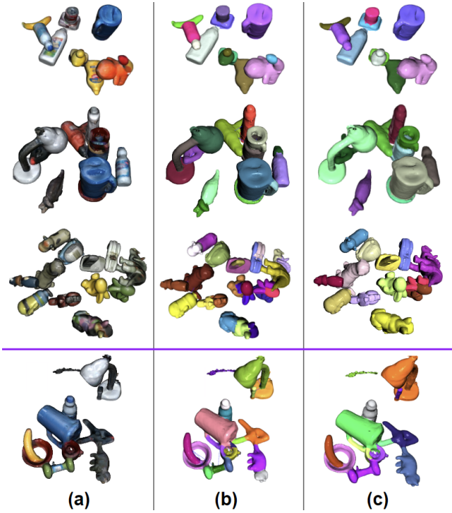
Fig. 6: Intermediate Qualitative 3D Segmentation Results (a) Reconstructed object point clouds in their original color. (b) Segmentation results from LCCP + SymSeg. (c) Object pseudo labels after graph matching and pruning given over-segmentation results as inputs. A failure case of over-segmentation is shown in the last row, where part of the “pitcher” and “cup” are not separated and the “cup” is segmented into inconsistent pieces. This cannot be addressed during graph matching.
