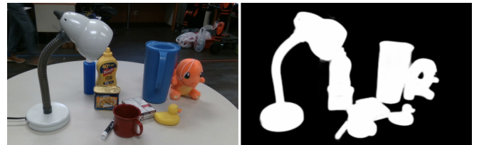
Fig. 2: Example of saliency detection [28] for generating the foreground mask (right) given RGB input (left).
