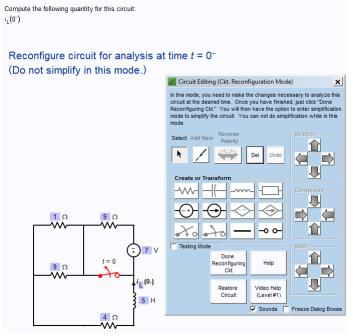
Fig. 1. Example of a first-order transient circuit being reconfigured prior to solution at  $t = 0^{-1}$ .
