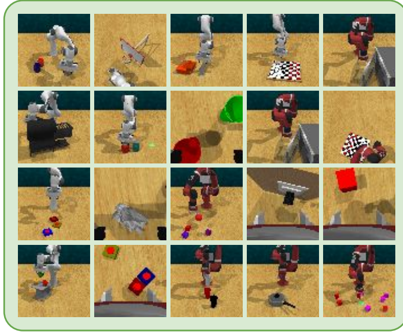
Figure 13: A single autoregressive video model is trained on 30 tasks for the Franka Panda and 23 tasks for the ReThink Robotics Sawyer, using 16 \times 16 VQCodes and a context length of 4, with frame skip 4.
