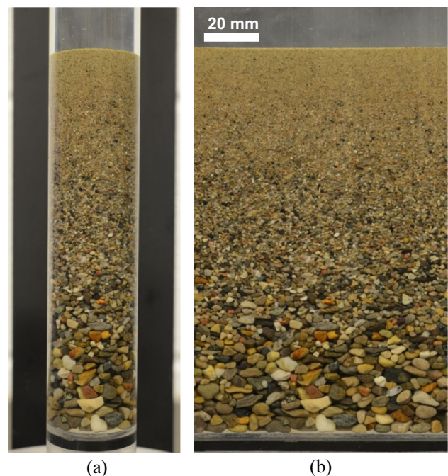
Fig. 2 Soil specimen in the Sed360. a Image captured during sedimentation column rotation, b Unwrapped view of the soil specimen perimeter
