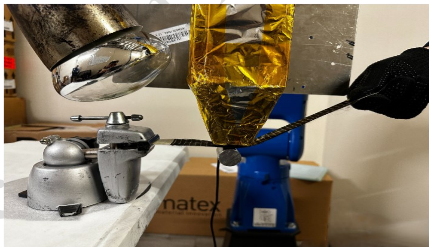
Figure 4: In this under-development robot-arm driven MCFA-AM printer, A carbon fiber tape is being hand-fed and held by a backing article (cylinder) attracted by a magnetic field emitter (wrapped with aluminum foil).
