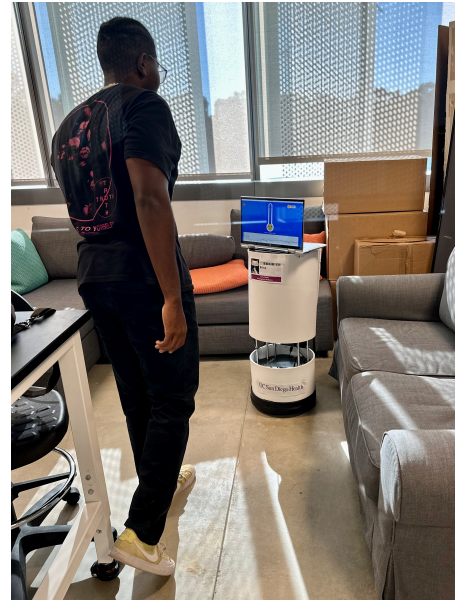
Figure 1: A user interacting with GARRY, an interactive robotic system that provides real-time feedback to users during locomotor training.
