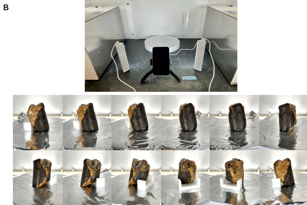
Figure F24. A. DMT CoreScan3 workstation with example of 3-D high-resolution image created using novel methods developed during Expedition 390. B. Foldio workstation with rotating stage and camera positioned to take multiple time-lapsed images of core pieces as it rotates that were taken to preserve information on pieces fragmented for microbiological sampling.
