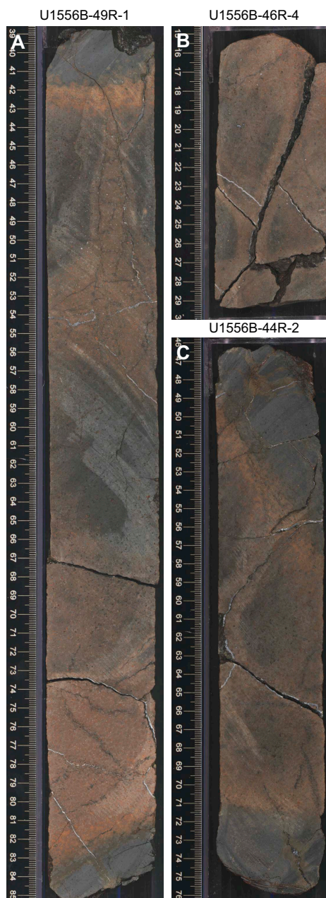
Figure F67. Well-developed orange halos that are almost pervasive at core scale, Hole U1556B. A–C. More intense orange coloration along veins and adjacent to margins. Some carbonate veins are associated with halos, whereas others are not, suggesting that growth of carbonate veins both accompanied and postdated halo formation.
