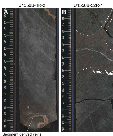
Figure F59. Typical examples of dark gray background alteration, Hole U1556B. A. Brownish sediment-derived veins are also shown. B. Faint orange halo with sharp rusty orange front along two carbonate veins with halo width approximately proportional to each of the vein widths.
