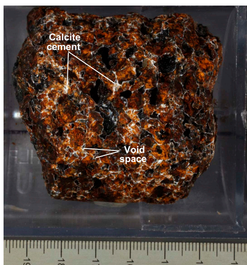
Figure F24. Calcite-cemented breccia with void spaces and relatively fresh glass (390-U1556B-13R-1 [Piece 4, 13–19 cm]).
