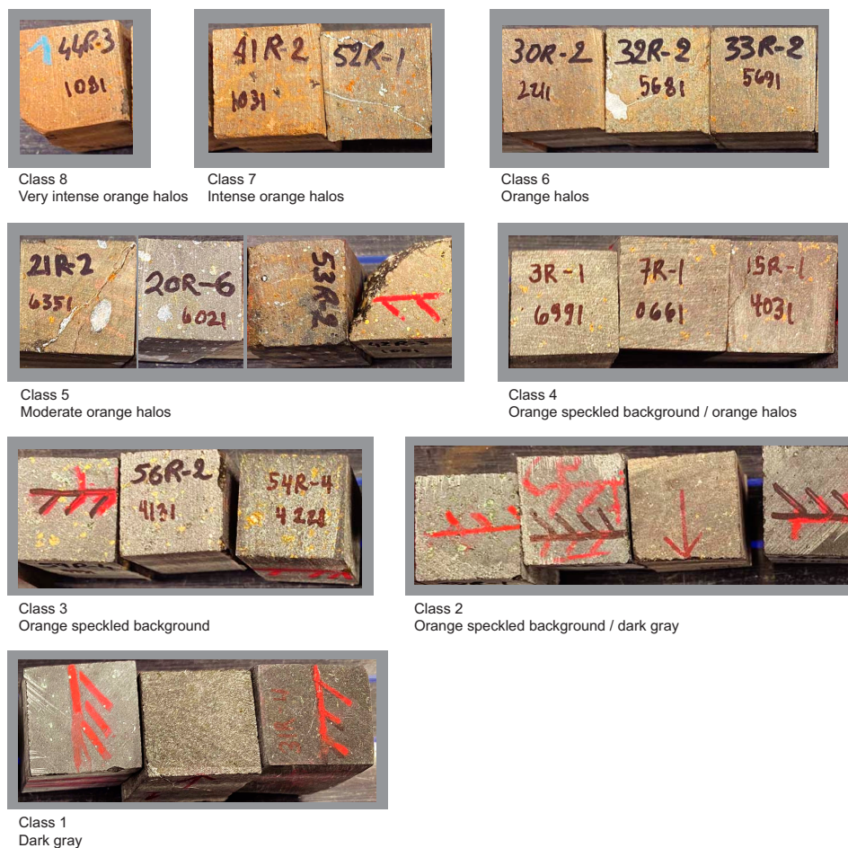
Figure F140. Examples of alteration classes assigned to discrete basalt samples, Hole U1556B. Alteration classes range from Class 1, characterized as dark gray, to Class 8, characterized by very intense orange halos (Table T27) (see Alteration petrology).
