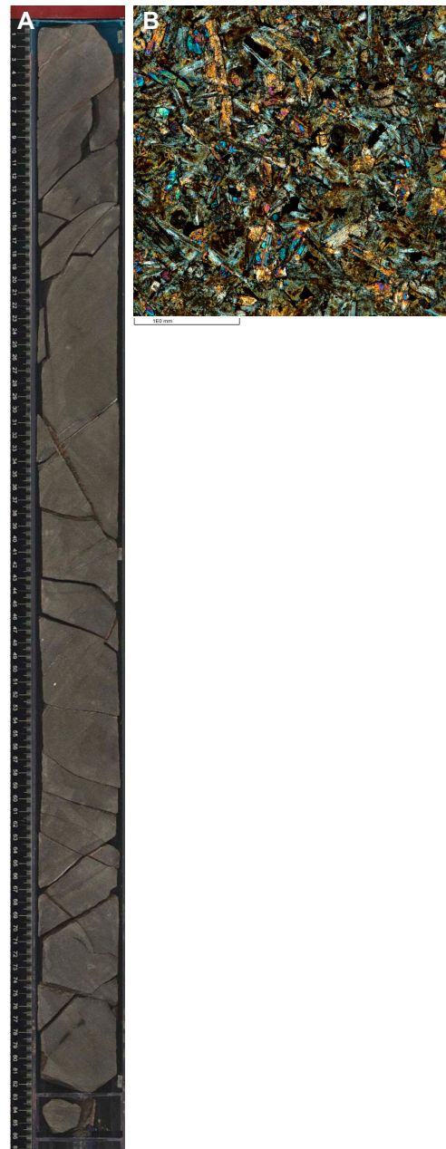
Figure F37. A. Massive interval in Unit 12 (390-U1556B-51R-1). Intense fracturing is typical of this lithology. B. Microcrystalline texture (51R-1 [Piece 1, 36–38 cm]). Compare with cryptocrystalline textures shown in Figure F34C–F34E.
