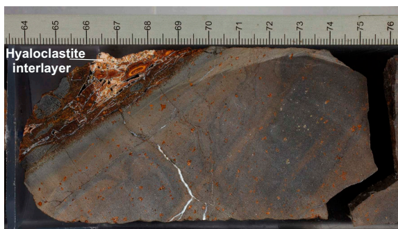
Figure F30. Orange spotty basalt with hyaloclastite interlayered within glassy chilled margin (390-U1556B-34R-1 [Piece 11, 64–76 cm]).
