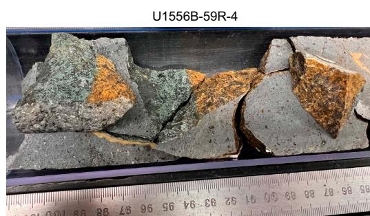
Figure F82. Sharp reaction/oxidation front between pale green clay and oxidized orange Fe oxyhydroxide-rich material along a vein, Hole U1556B. Front is present throughout the rock and marks boundary between meters-thick interval of dark green background alteration above and orange speckled background alteration below.
