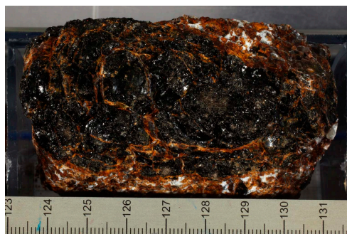
Figure F23. Fresh glass in hyaloclastite (390-U1556B-12R-3 [Piece 19, 123–132 cm]).
