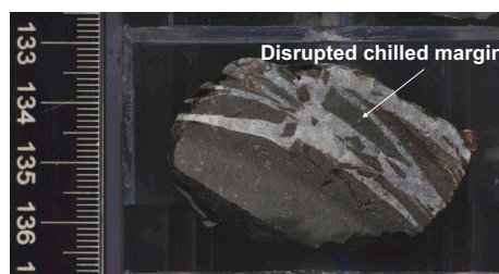
Figure F21. Hydrothermal fracturing of chilled pillow margins and formation of one style of hyaloclastite, Hole U1556B (11R-1 [Piece 11, 133–137 cm]).
