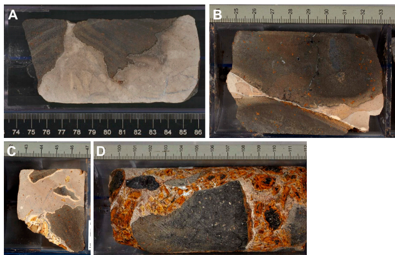
Figure F17. Sedimentary breccia, Lithologic Unit 1. A. Subunit 1a (390-U1556B-2R-2 [Piece 5, 75–86 cm]). B. Subunit 1a (390-U1556C-32X-1 [Piece 6, 25–33 cm]). Note there are at least two generations of sediment, one pale brown, disrupted by a vein created by whiter sediment being squeezed up between two basalt clasts. There are also fragments of a third sediment, whiter in color, adhering to side of basalt clast at bottom of image. C. Sedimentary breccia in Subunit 1a showing whiter sediment adhering to clasts floating in pale brown sediment (32X-1 [Piece 8, 42–47 cm]). D. Hyaloclastite-like matrix in Subunit 1b rich in altered glass clasts (32X-1 [Piece 13, 99–111 cm]).
