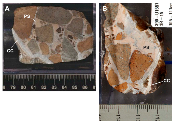
Figure F22. Sparry calcite vein, Subunit 1b. A. 390-U1557D-3R-1 (Piece 4, 79–85 cm). B. 3R-1 (Piece 6, 105–111 cm). PS = pelagic sediment, CC = calcite cement.
