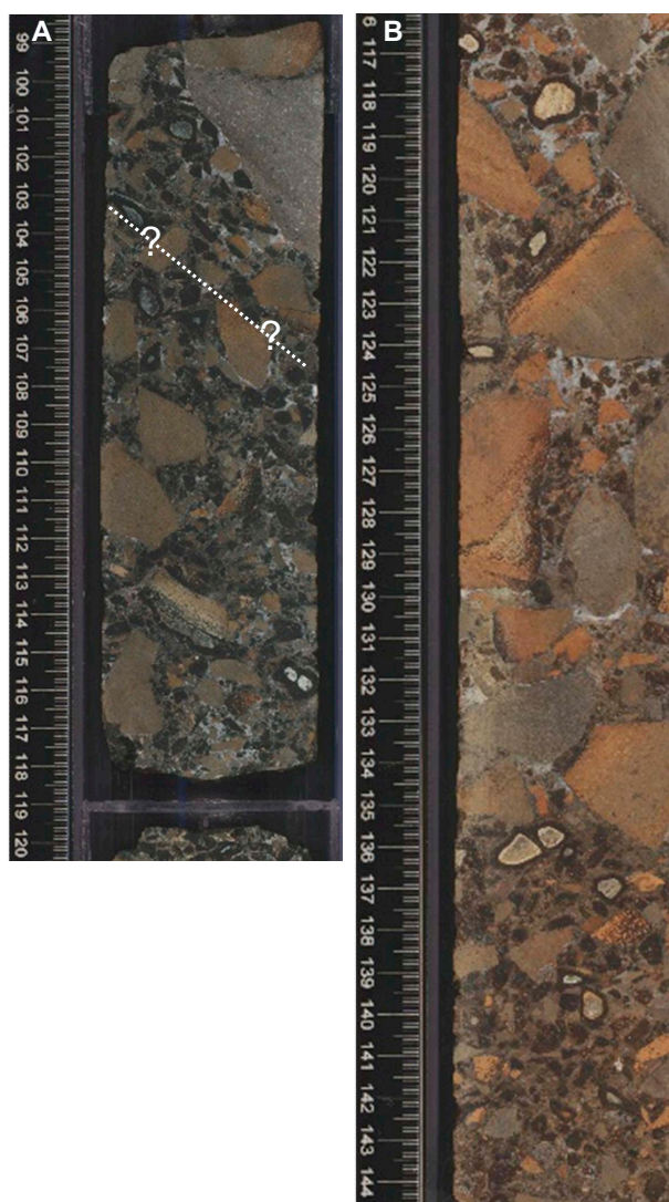
Figure F30. Increase in compaction toward bottom of Hole U1557D. A. 10R-1, 99–118 cm. White dashed line = possible preferred alignment of clasts created by compaction and/or deformation. B. 10R-2, 116–144 cm. See Figures F16, F20, F21, F22, and F25 for examples of rock textures higher in hole.
