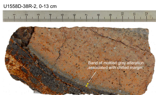
Figure F41. Mottled gray chilled margin alteration showing narrow (3–4 mm) band of gray alteration between glassy margin and pillow interior that is altered to orange halo.
