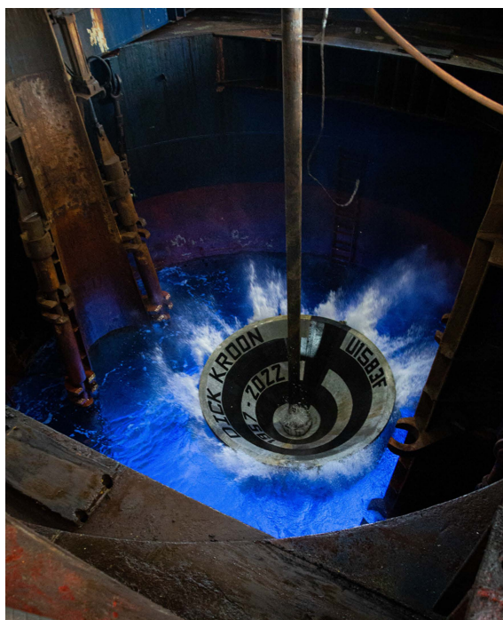
Figure F5. Launch of a free-fall funnel, named in honor of Professor Dick Kroon, Hole U1583F (Credit: Erick Bravo, IODP JRSO).
