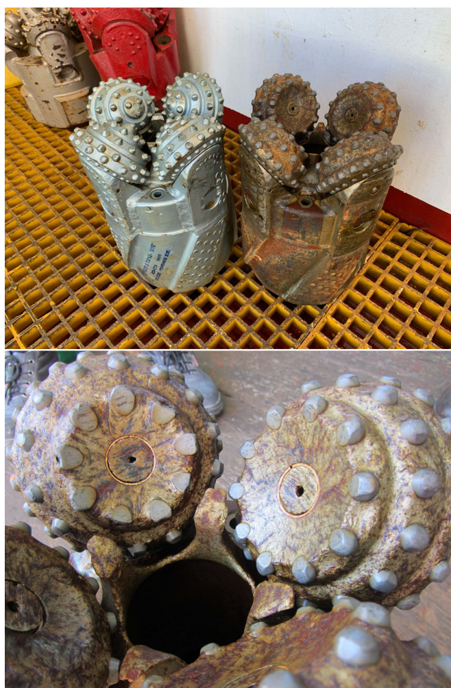
Figure F6. Top: Drill bit used to core Hole U1559B (right) in comparison to fresh drill bit (left). Bottom: Close-up of wear on roller-cones and core guides. Note extensive damage to roller cones.
