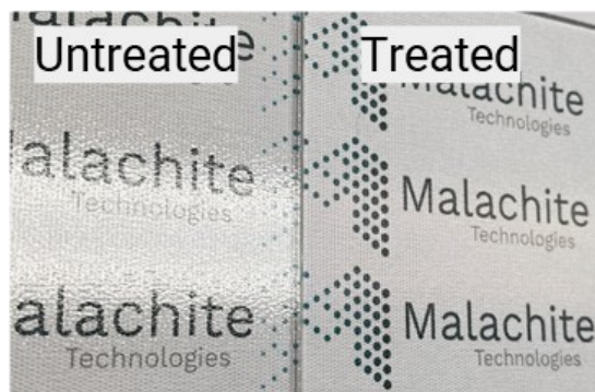
Figure 6. Image comparing visual reflectance change of treated vs untreated low-Fe glass used for solar applications.
