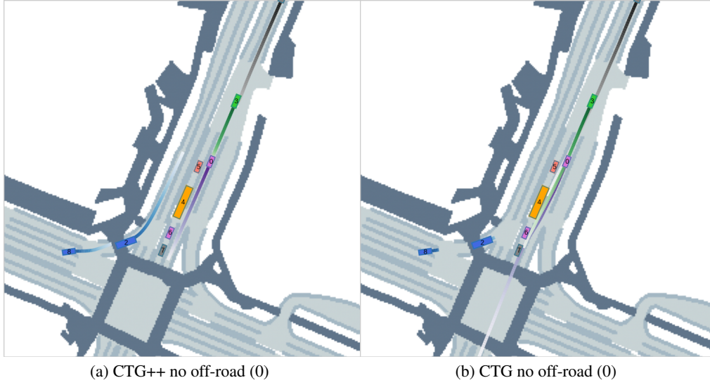
Figure A5: Qualitative comparison between CTG++ and CTG under no off-road STL rule (the numbers in parentheses represent rule violations). Both methods satisfies the rule perfectly as no off-road happens. However, CTG lead to multiple collisions among the pink vehicle and vehicles that are stationary.
