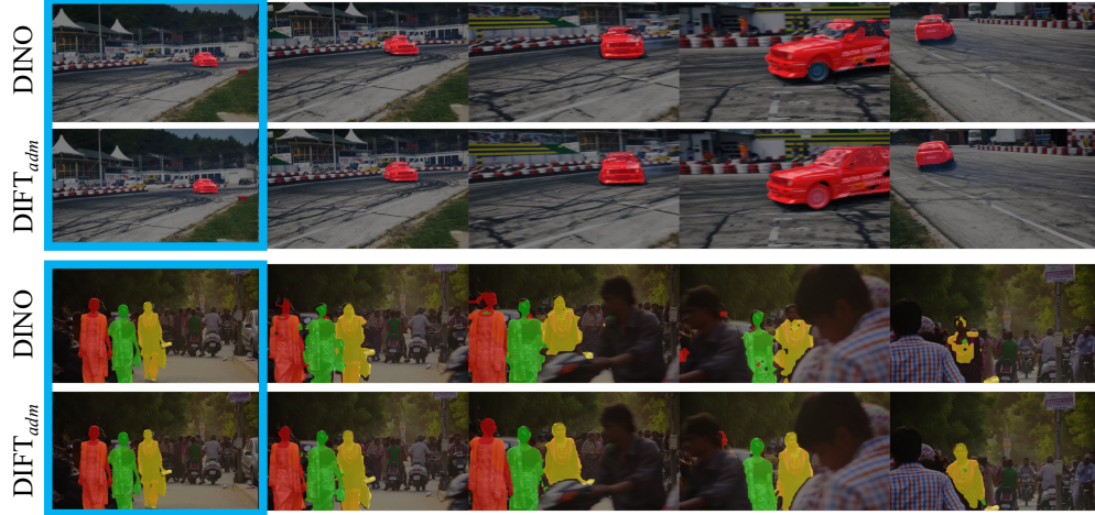
Figure 8: Video label propagation results on DAVIS-2017. Colors indicate segmentation masks for different instances. Blue rectangles show the first frames. Compared to DINO, DIFT adm produces masks with more accurate and sharper boundaries. More results are in Fig. 22 of Appendix E.
