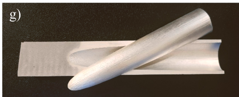
Fig. 16. Shear test fracture morphology. The samples were extracted from the AA6061 round bar, single-piece billet extrusion, with butt shear (except where specified otherwise).
