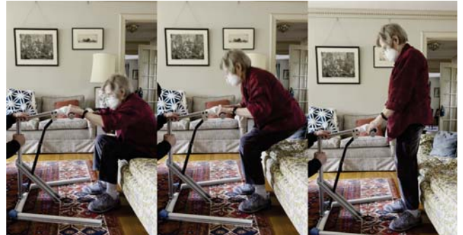
Fig. 1. An elderly subject performing a sit-to-stand transition using the handlebar manipulandum. Photo included with consent.
