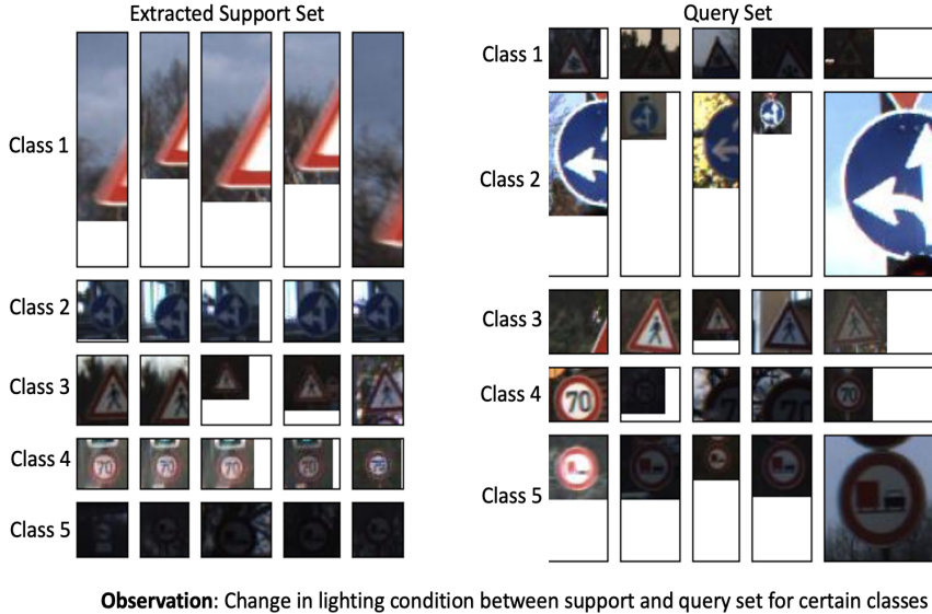
Figure 32: Difficult Task from Traffic-Sign: This extracted task from traffic_sign has an accuracy of 15%. We find that this task has a distribution shift between the support and query with respect to various lighting conditions. For e.g., Class 5 in the extracted support set has almost no light when compared to the images from Class 5 in the query set.
