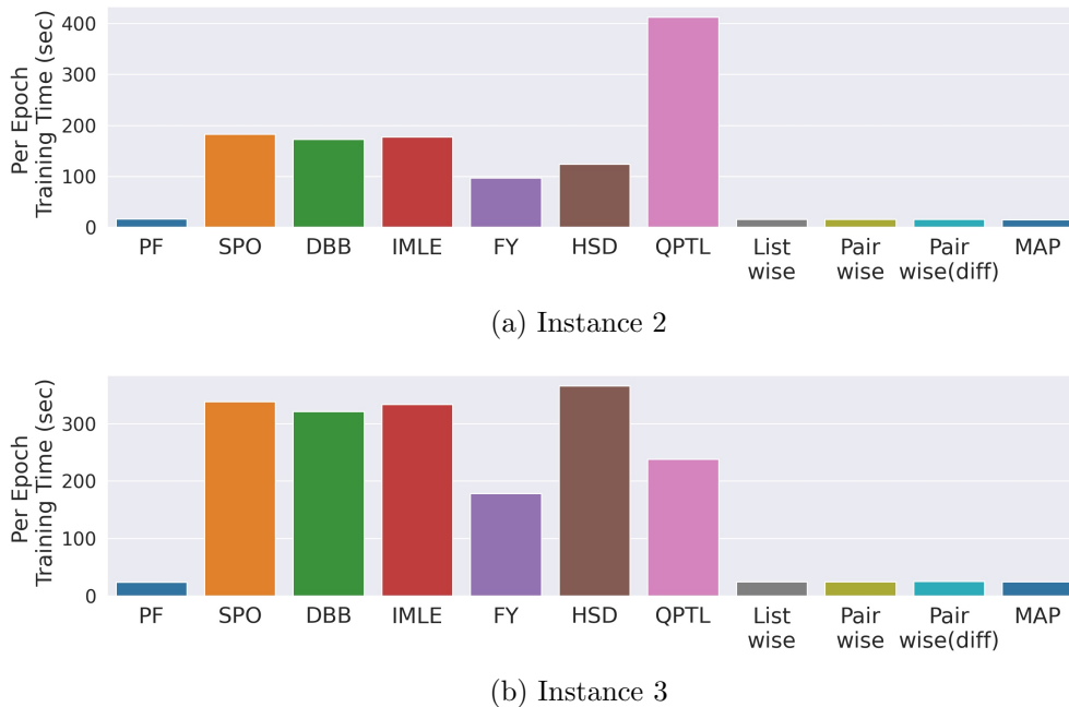
Figure 12: Comparative evaluations of per epoch training time of different DFL methodologies on the energy-cost aware scheduling problem.
