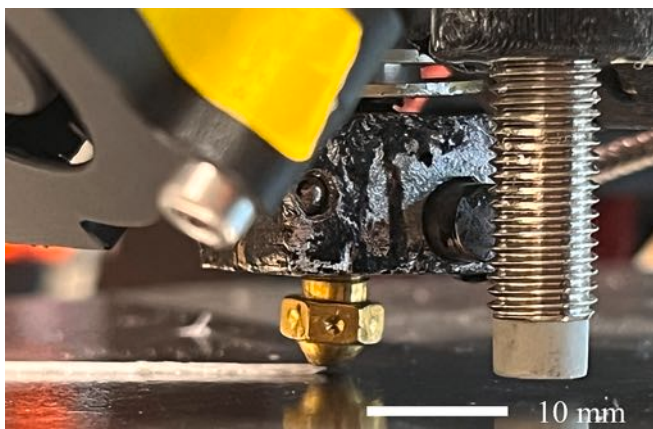
Fig. 2. Printing of 0.8 mm filament with dispersed fibers using a 1.2 mm brass nozzle.
