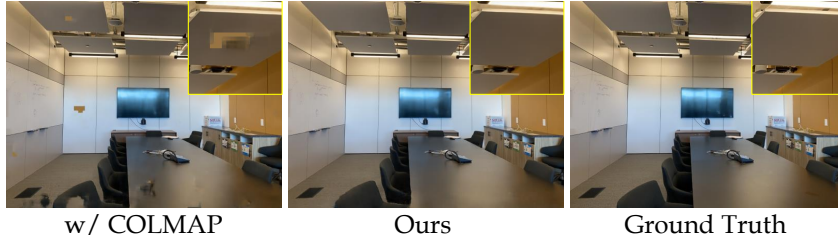
Figure 9: We visually compare the results of using the COLMAP fused point cloud against our proposed MVS finetuning + point sculpting. Our point cloud has higher completeness and thus better visual quality, especially in texture-less areas (e.g., the zoomed-in ceiling region).
