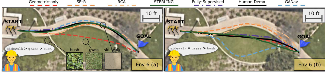
Figure 6: Trajectories traced by different approaches for the task of preference-aligned off-road navigation. Shown here are two different preferences expressed by the operator in the same environment—in 6 (a), sidewalk is more preferred than grass which is more preferred than bush, and in 6 (b), grass and sidewalk are equally preferred and bush is least preferred. We see that without retraining the terrain features, in both cases (a) and (b), STERLING optimally navigates to the goal while adhering to operator preferences.
