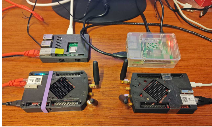
Fig. 4: Hardware setup for performing interoperability between two Red Pitayas.
