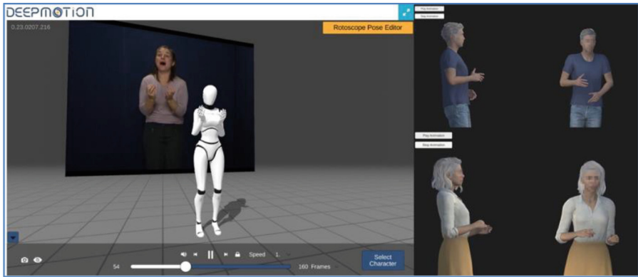
Fig. 1. Left: screenshot from video-based motion capture software showing the video of the actor in the background and the extracted gesture applied to a 3D mannequin in real-time. Right: frames extracted from two of the animation stimuli.
