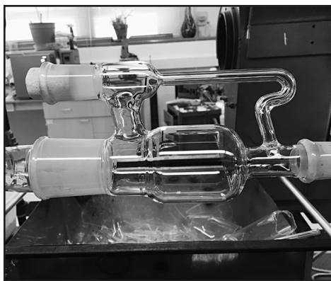
Figure 11. Completed pyrolysis chamber body
