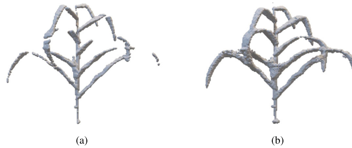
Fig. 16. A comparison between results of traditional voxel carving and probabilistic voxel carving algorithms. The resolution is set as resX = 256 and the dilation \delta = 2 . The plant we show here is Sample 1. (a) The result of the traditional voxel carving algorithm. A lot of disconnections can be spotted in the output model. (b) The result of the probabilistic voxel carving algorithm with the threshold \tau = 0.8 .
