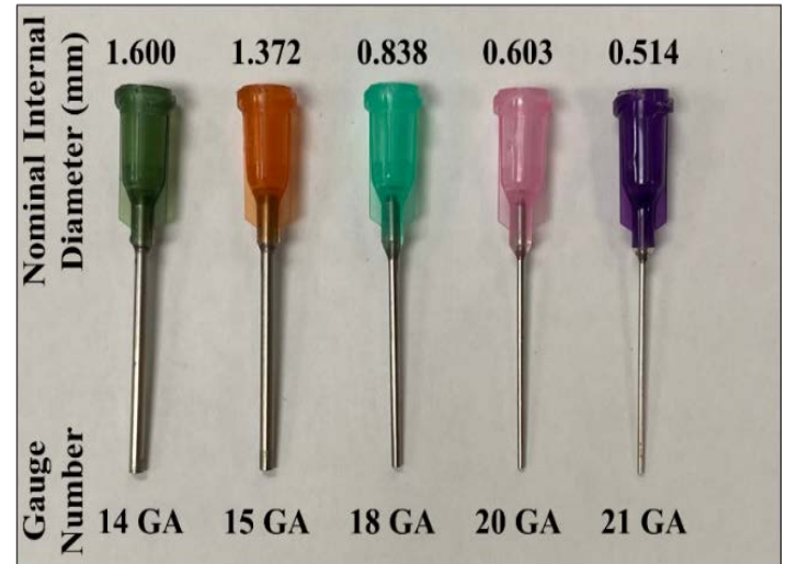
FIGURE 1: SIZE COMPARISON OF NEEDLE GAUGES USED TO PRODUCE WATER DROPLETS.
