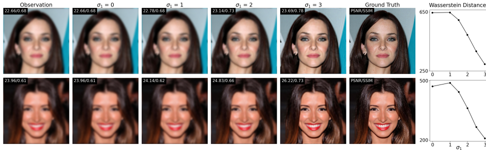
Figure 4: Illustration of the PnP-ULA stability to a mismatch forward model. Leftmost six plots: MMSE estimators computed with PnP-ULA run on 30,000 steps on Gaussian blur of standard deviation \sigma_1 . Rightmost: Evolution of the Wasserstein distance between sampling distributions computed with a mismatched blur kernel, \sigma_1 \in [0, 3[ and sampling with the exact forward model \sigma^* = 3 . Note that the image reconstruction quality improves as \sigma_1 gets closer to \sigma^* = 3 , used to degrade the image. In addition, in the case of Gaussian blur, the pseudometric is given by |\sigma_1 - \sigma^*| which justifies qualitatively the observed linear decrease of the Wasserstein distance.
