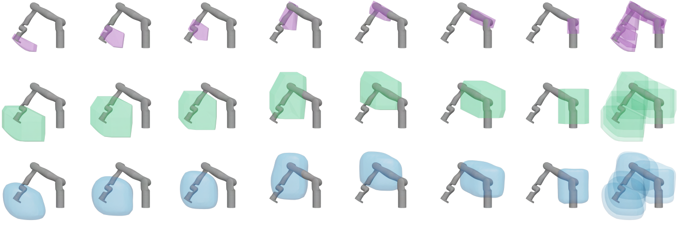
Fig. 3: 3D Reconstruction of RDF's zero-level sets compared to Alg. 1. (Top) Convex hull of each link's forward occupancy reach set (purple) before buffering by obstacle generators (Alg. 1, line 6). (Middle) Following buffering, the size of the new forward occupancy (green) is increased (Alg. 1, line 7). (Bottom) RDF's zero-level set (blue) is shown to be a smooth approximation to that of the convex hull buffered forward occupancy reach set (middle, green).
