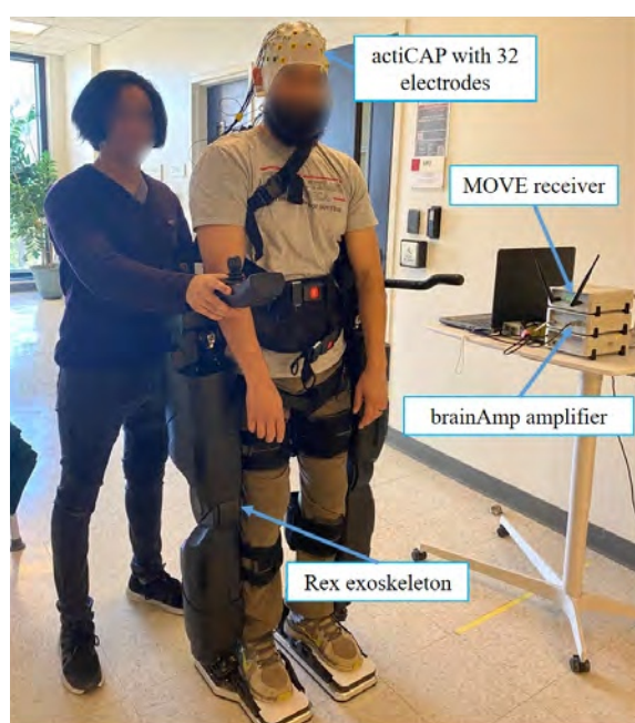
Figure 1. Equipment used in the protocol.
