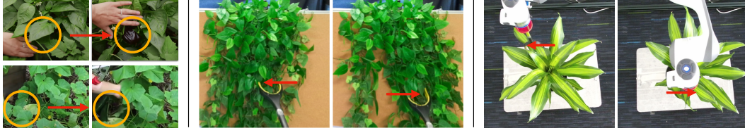
Figure 1: (left) Plants self-occlude themselves. Two examples of leaves and branches being pushed aside for inspection and picking fruits. This paper develops learning algorithms that enable robots to tackle this plant self-occlusion problem. We show actions executed by the robot to expose the space behind vines (middle) and Dracaena plant (right) .
